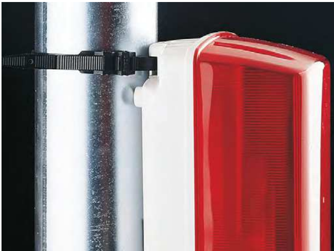
MIZAR Series MIZAR Series light-fittings are fitted with a slot on the rear of the base for hooking onto a nail, screw or hook, or for fastening to poles, pipes, bars or scaffolding using one or two cable ties.
